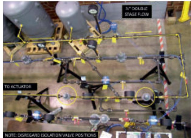
Figure 4. Close-up showing flow from reservoirs through 1/2" double stage flow circuit
