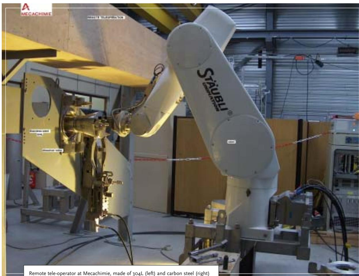
Remote tele-operator at Mecachimie, made of 304L (left) and carbon steel (right)
