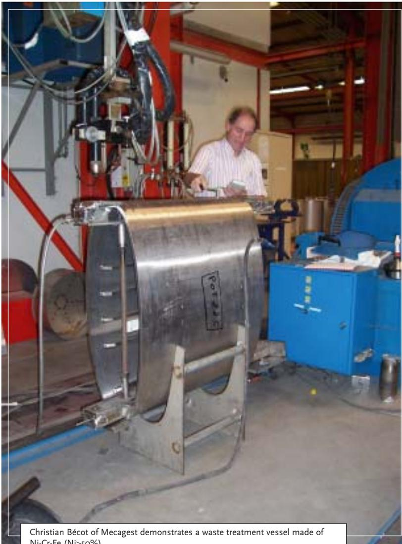
Christian Bécot of Mecagest demonstrates a waste treatment vessel made of Ni-Cr-Fe (Ni > 50%)
