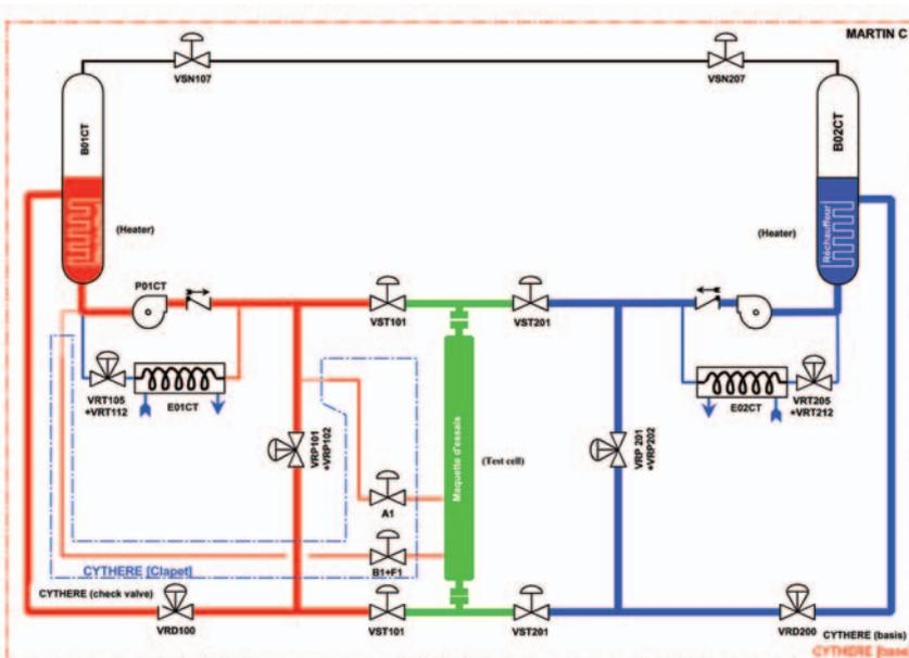
Figure 2: The CYTHERE test facility scheme
