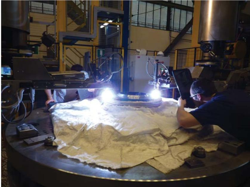
*Figure 3. Buttering process for welding of buffer layers to prepare joints of homogeneous, dissimilar materials.*
