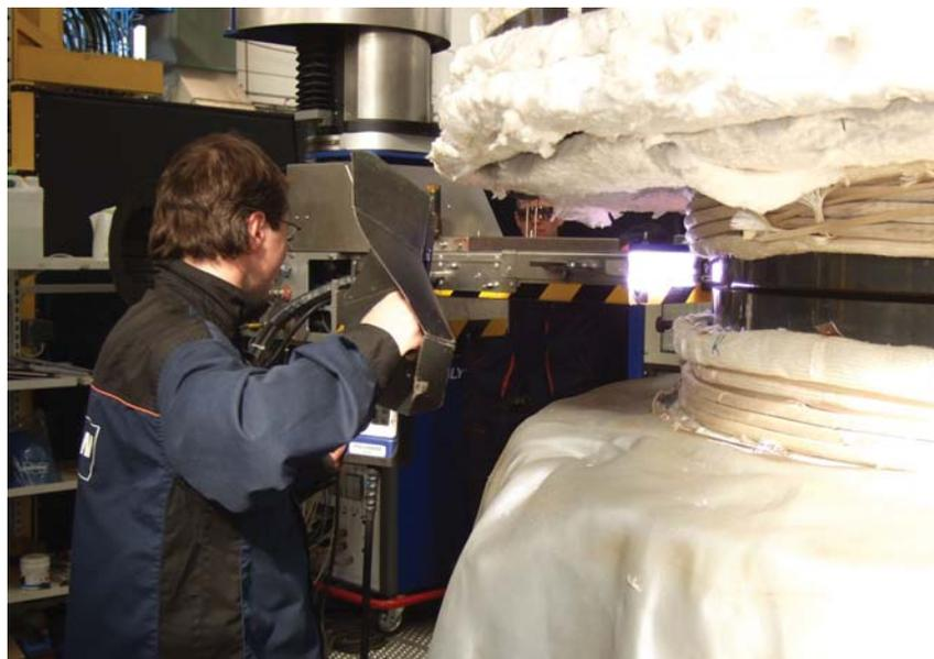
*Figure 4. One of the eight specially trained welders controls the progress of a nearly finished weld; here the conventional TIG torch is installed.*
