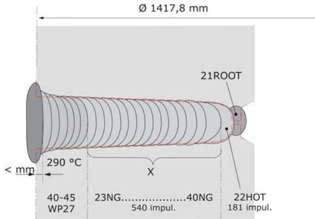
Figure 7. Disposition of welding passes. 21ROOT = root pass 180° (x 2); 22HOT = hot pass 180° (x 2); 23NG – 39NG = filler passes with narrow gap torches 540° (x 2); 40WP27 – 45WP27 = filler passes with conventional TIG torches 540° (x 2).
