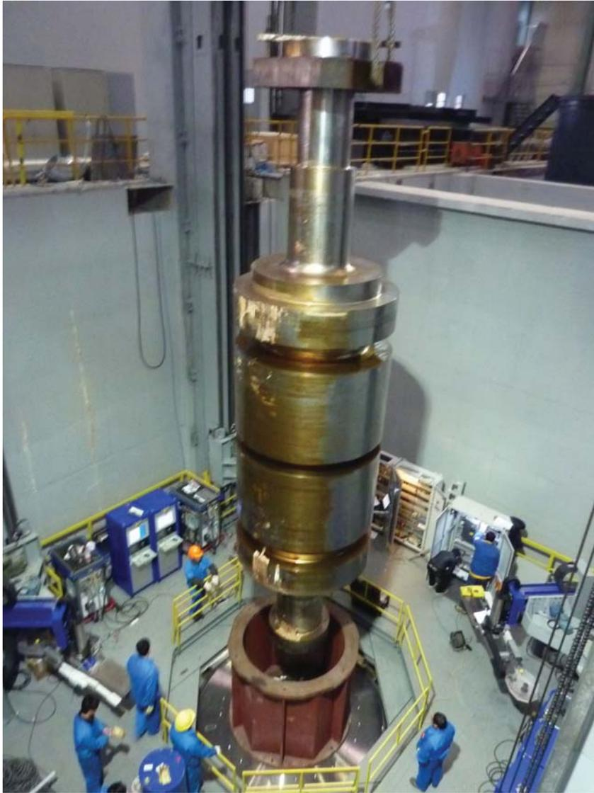
Figure 1. TIG welding station for joining vertically positioned rotor Parts.
