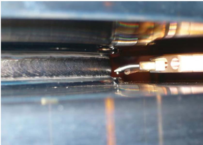
Figure 6. Narrow groove with introduced torch after root pass has been welded.
