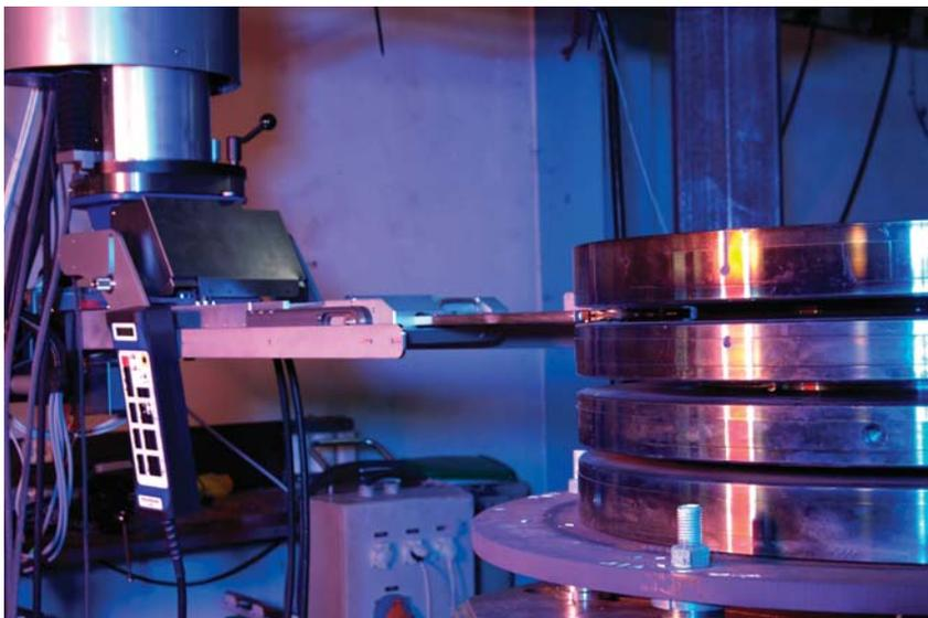
Figure 2. Horizontal arm support and installed narrow gap TIG torch.
