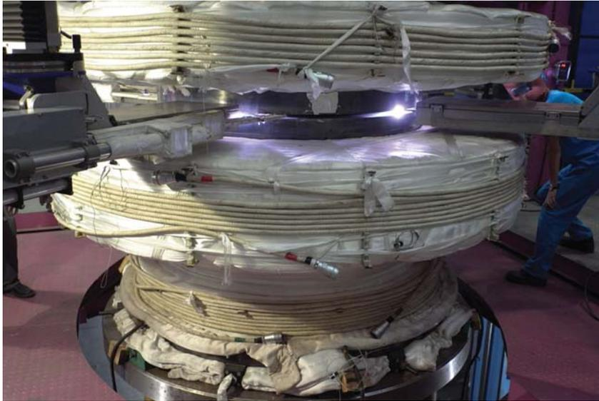
Figure 5. Welding of specimen for process qualification at the Polysoude welding application department, with two narrow gap TIG torches in opposing positions.
