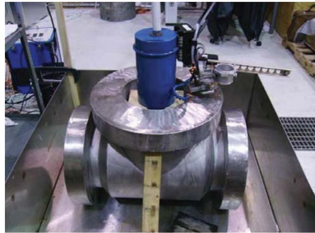
Figure 2. Photographs showing manual and automated inspection of the valve body in process.
