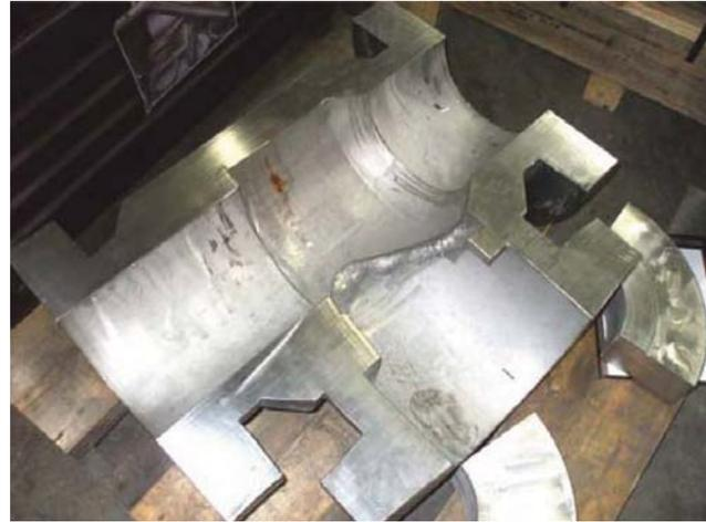
Figure 1. A 780kg (1716 lbs), 316L prototype stainless steel valve body produced during the feasibility assessment. The valve body was sectioned along its center line to reveal its ability to produce a sound, dimensionally stable, component configuration.
