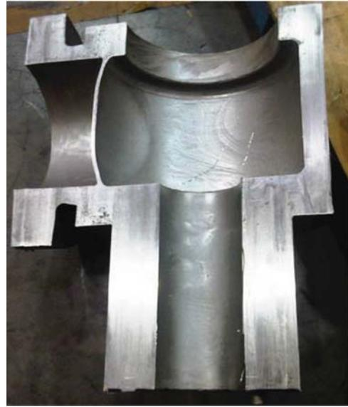
Figure 4. Three Grade 91 alloy steel valves (such as the one on the left) were manufactured by Carpenter Technology to drawing/specifications provided by Dresser. The valve body shown on the right of the first photograph is manufactured from IN625. The figure on the right shows a Grade 91 valve body that is sectioned into two halves.
