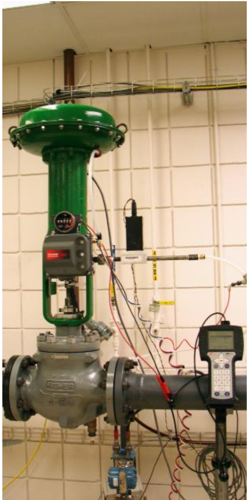
Pressure control mode test setup
