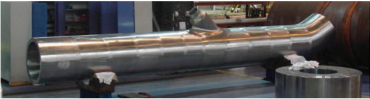
Figure 3. Example of a forged leg with integrated nozzle and elbow.
