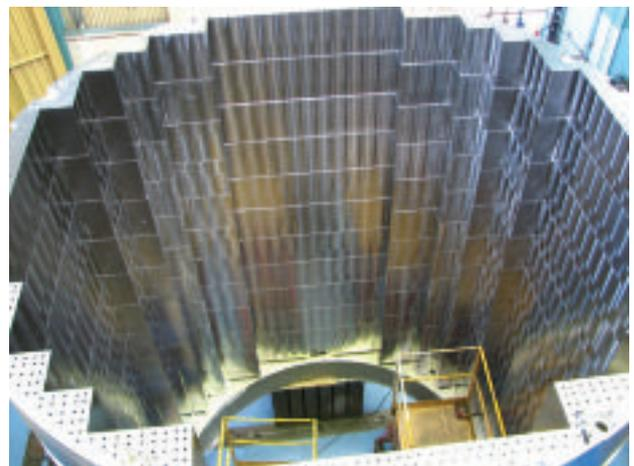
Figure 2. Lower internals for the EPR™ reactor (heavy reflector).
