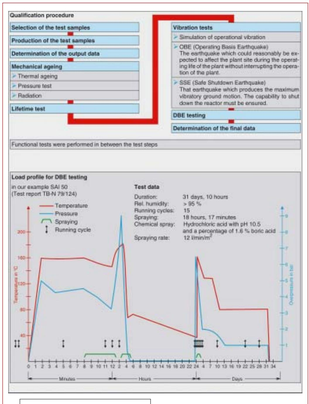
Figure 6: LOCA test for the multi-turn actuator SAI
