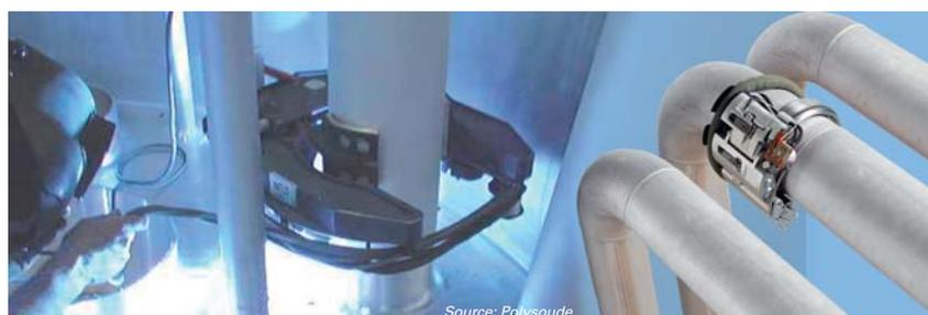
Fig. 1. Complex piping systems in a uranium enrichment facility welded using a Polycar 30 low profile open carriage-type welding head.
