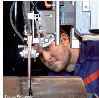
Fig. 3. Safe-end flange welding.
