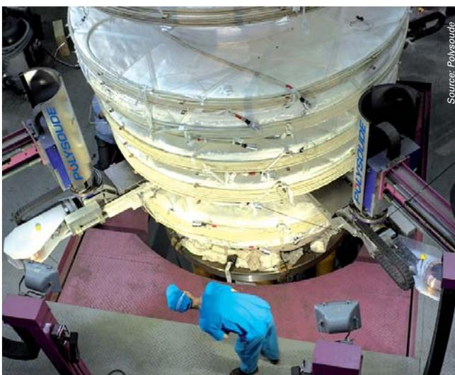
Fig. 5. TIG welding station for joining vertically super positioned rotor segments.
