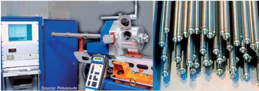
Fig. 2. Precision vacuum welding lathe for high alloy steel end caps.
