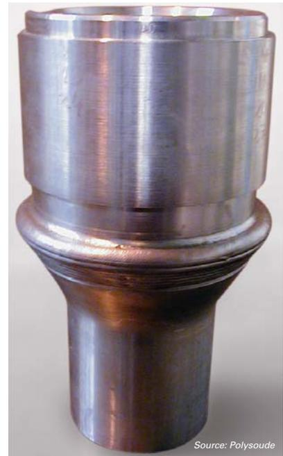
Fig. 6. Canopy joint rebuild.
