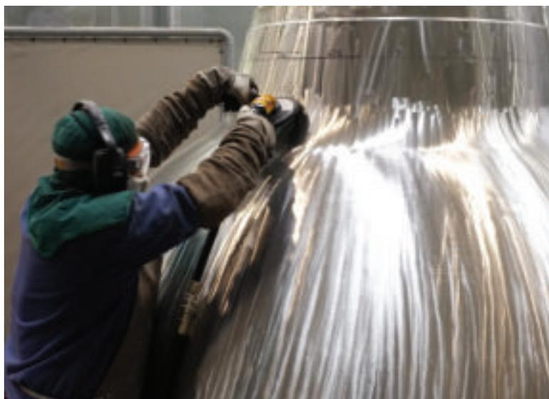
Grinding of a main reactor cooling pump before dispatching.
