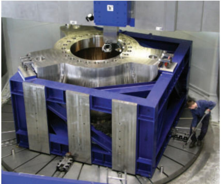
*Main reactor cooling pump during final machining.*
