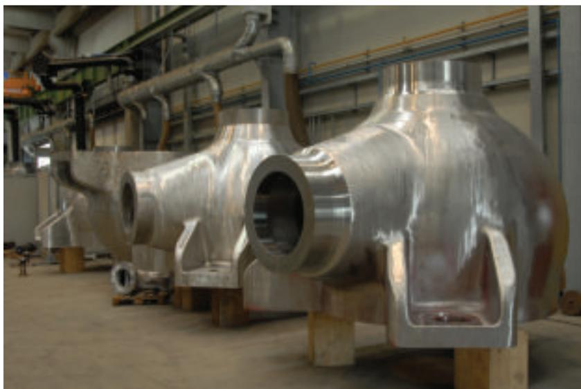
Main reactor cooling pumps during manufacturing at Safas.
