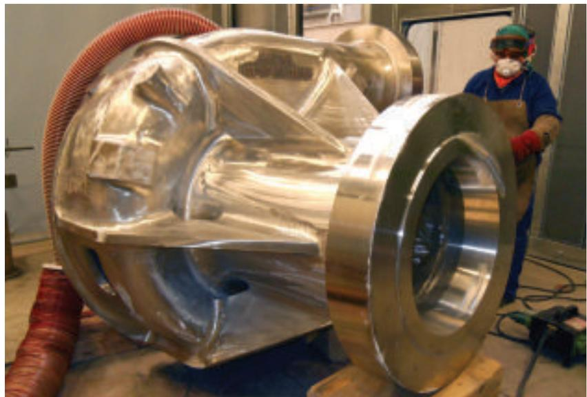
*Main reactor cooling pump of Cadarache (reactor Jules Horowitz).*
