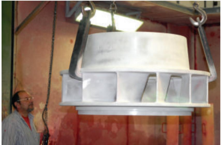
*Penetrant test on a diffuser of primiry circuit.*
