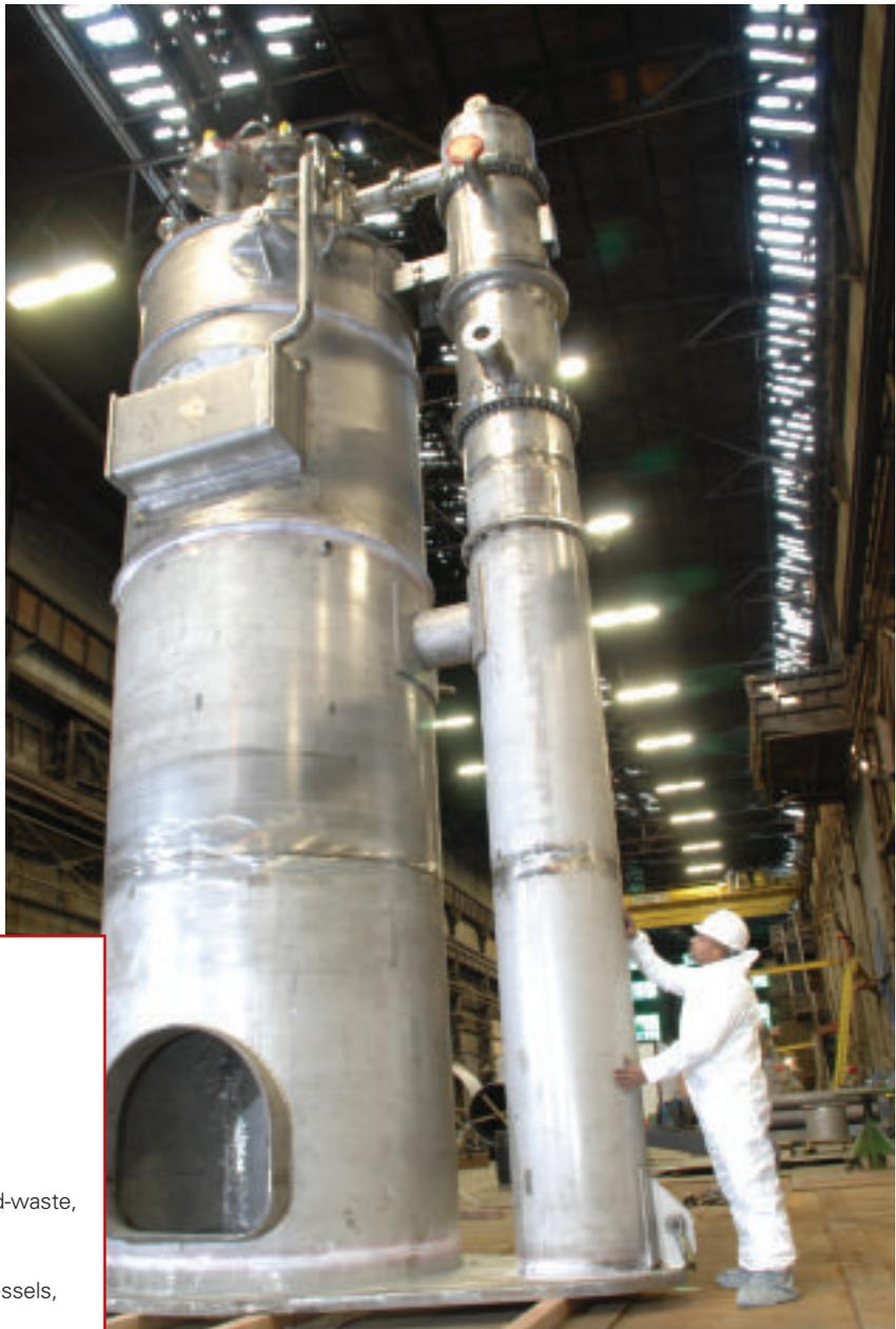
*A high nickel alloy pressure vessel being prepared for the US Department of Energy.*
