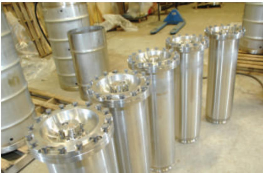
*Canisters for the storage of radioactive waste, fabricated as part of the company’s ‘legacy clean up’ activities with the US Department of Energy.*
