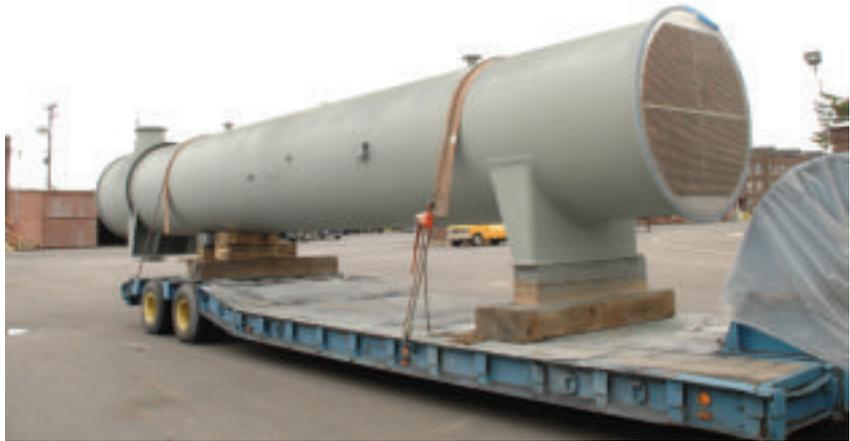
*Joseph Oat manufactures ASME Section III and Section VIII Component Cooling Water (CCW) Heat Exchangers for nuclear utilities from a variety of tube materials, including copper nickel, 6 moly stainless steel and titanium. A large CCW HX is shown completing a visit to the paint booth.*
