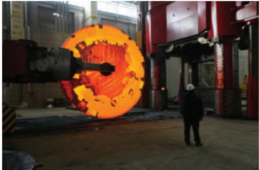
*Tube sheet being prepared at the FOMAS plant in Italy.*
