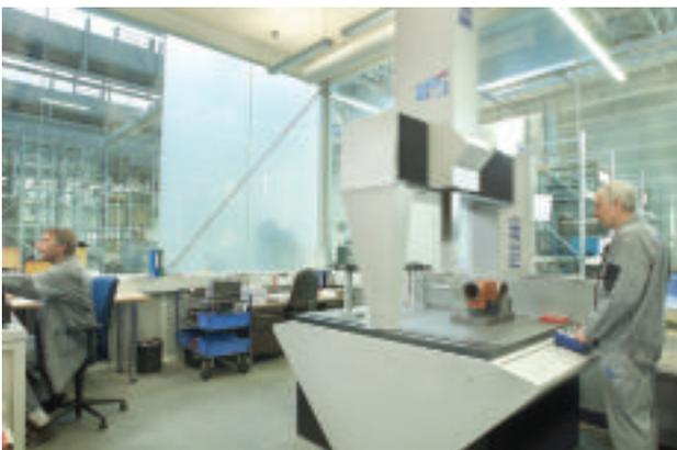
*High precision dimension check of actuator housing.*
