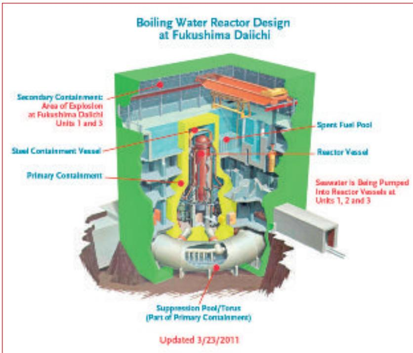
Figure 3. Boiling Water Reactor, Mark-I similar to D1, U1-5. D1, U6 is a Mark-II type. (Cf. www.nei.org)
