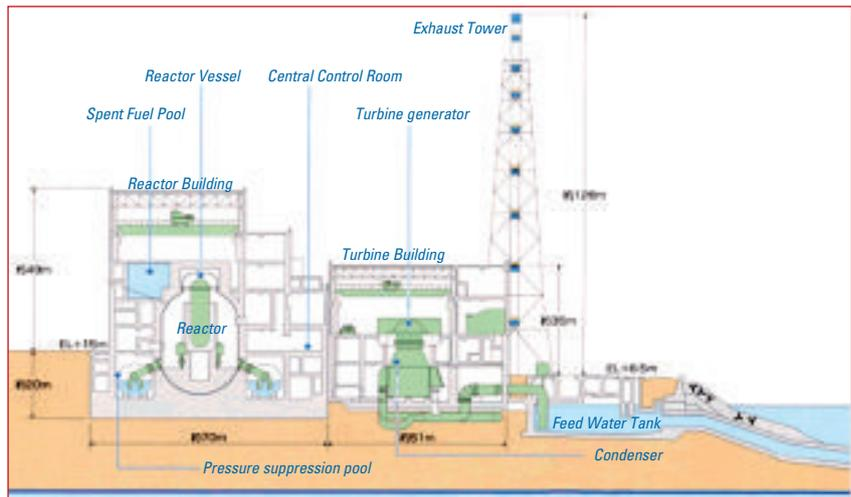
Figure 5. Representative cross-sectional perspective of D1 Unit (not all details are shown)
