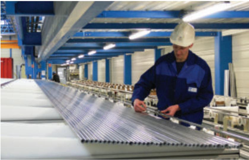
Valinox Nucléair's alloy 690 steam generator tubes are installed in power plants around the globe.
