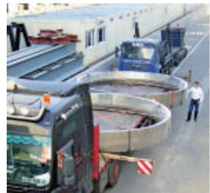
Skirt rings for pressure vessels prepared for transport
