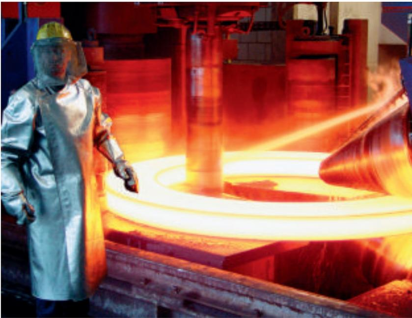
Ring rolling in progress at BRÜCK's Saarbrücken facility.
