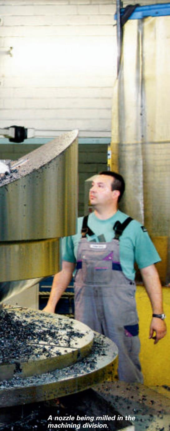
*A nozzle being milled in the machining division.*
