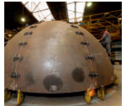
*A large vessel head manufactured using the crown and petals technique*
