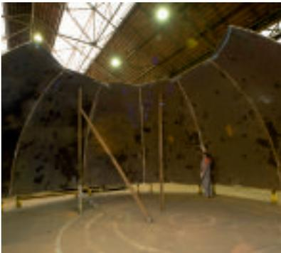
*Welders preparing the internal surface of a large vessel head manufactured using the crown and petals method.*
