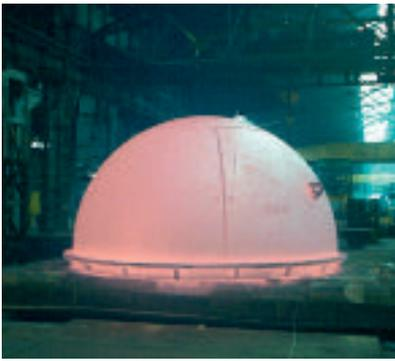
*A hot formed vessel head cooling in the company's production facility in Recquignies, France full stop.*
