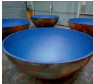
*Hemispherical vessel heads, painted with a protective blue coating on the interior surface, ready for shipping.*
