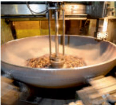
*Cold spinning a vessel head to prepare the edges for welding.*
