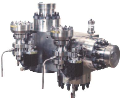
*The Sevim Tandem design is an innovative concept for over-pressure protection in the cooling circuit, incorporating two independent pilot-operated safety valves housed in the same body. The first valve ensures pressure safety and relief, while the second valve provides fail safe protection in the event of a failure of the primary valve, to significantly reduce accidental coolant loss.*
