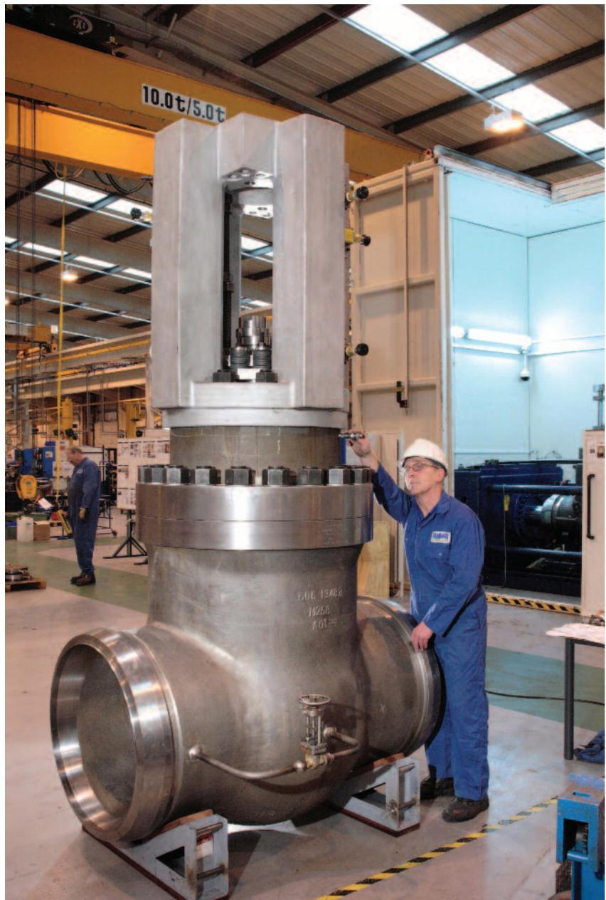
*At 5 meters tall and 750mm in diameter, the Main Steam Isolation Valves supplied to the Qinshan Nuclear Power Station Phase II Extension Project, are the largest Weir has manufactured at its Elland (UK) plant.*
