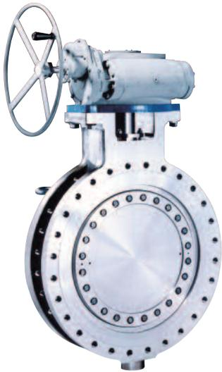
*The Tricentric® triple offset metal seated butterfly valve is installed on various nuclear applications, including containment isolation and service water systems. The torque seated design removes position seating concerns and the non-interference seat and seal design eliminates binding wear and tear.*
