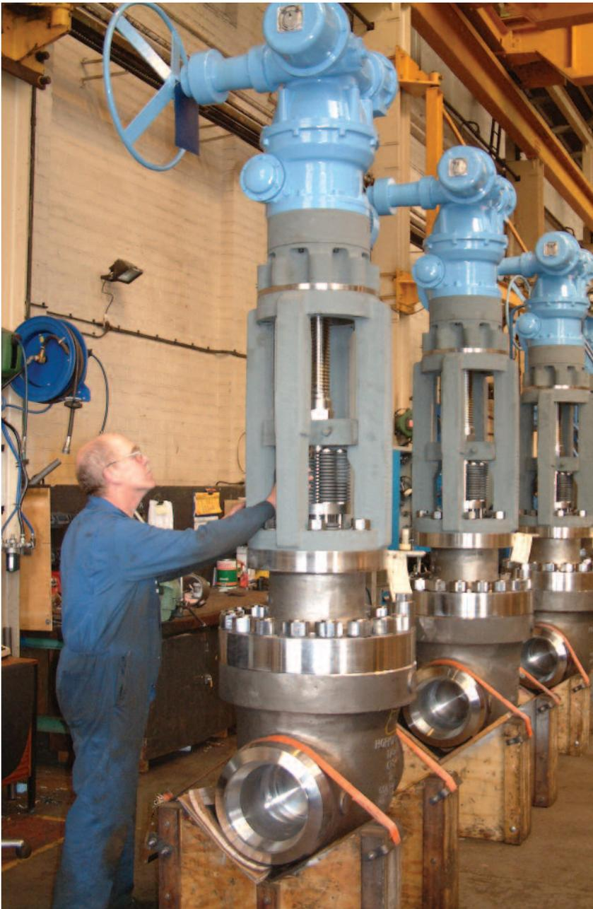
*Hopkinsons parallel slide gate valves undergoing final checks at the Elland (UK) plant.*
