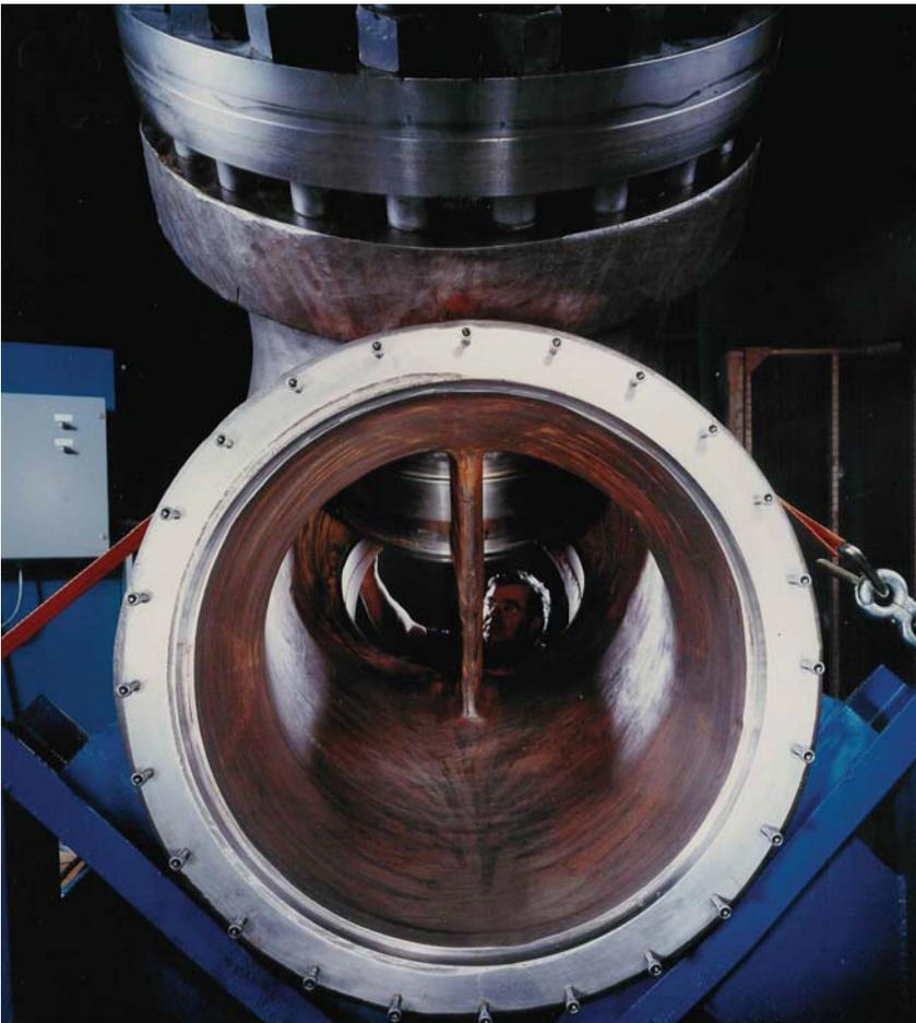
*Atwood & Morrill Wye Globe MSIV being prepared for testing. View shows the almost straight through flow passage*
