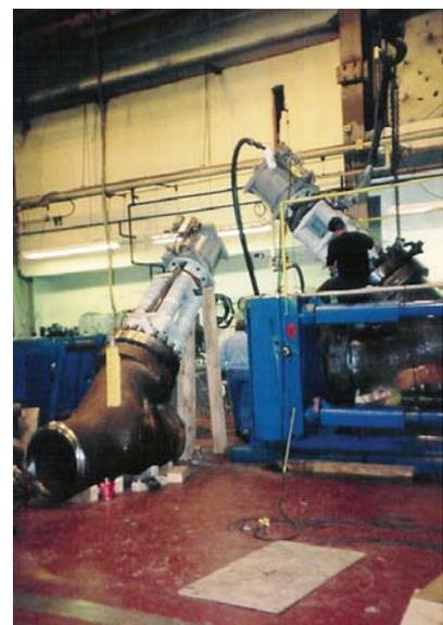
*WVC assembly and testing of Main Steam Isolation Valves in Salem facility*
