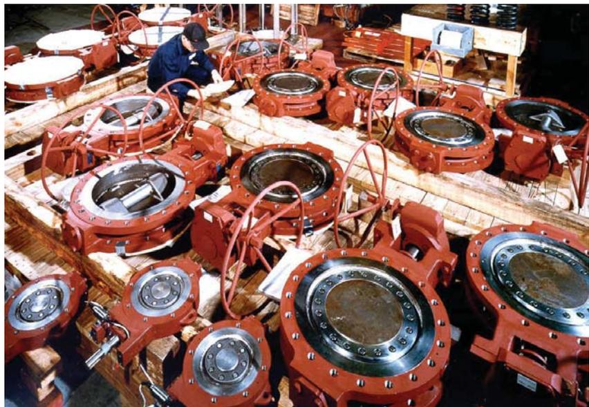
TRICENTRIC metal seated butterfly valves for service water applications in Lungmeen ABWR in Taiwan
