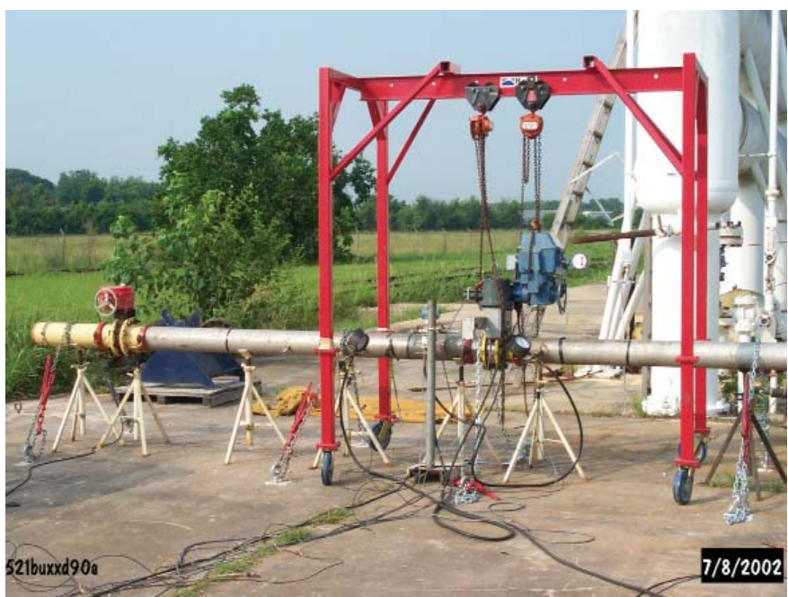
Compressible flow valve testing to precisely measure valve requirements for a variety of quarter-turn valve designs over a range of operating and installation conditions.
