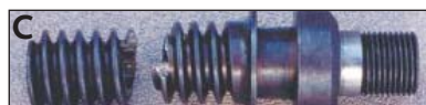
A: Coupled FEA and CFD model of a gate valve used to resolve pressure locking and thermal binding (PLTB) concerns. B: Testing to validate the predictive PLTB model C: Fatigue failure of motor operator worm that is accurately predicted using LiFE™ software
