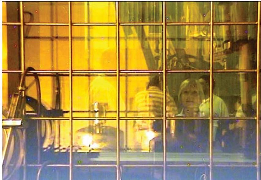
*Jan is treated to a demonstration of her client’s robotic arm, equipped with high rad camera as her picture is taken through the 18 inch leaded glass of a hot cell.*
