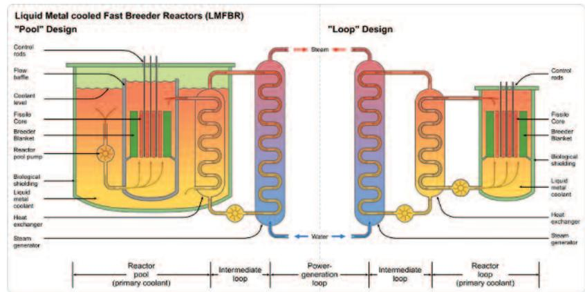
The “pool” and “loop” designs of a fast breeder reactor. In the loop design, all the components are contained in separate systems for ease of maintenance (as with PWRs). In the more compact pool design, all the primary reactor components are submerged in the reactor’s sodium pool, so that less radiation is released. From [upload.wikimedia.org/wikipedia/commons/8/85/LMFBR\\_schematics.png](http://upload.wikimedia.org/wikipedia/commons/8/85/LMFBR_schematics.png) Designs.
