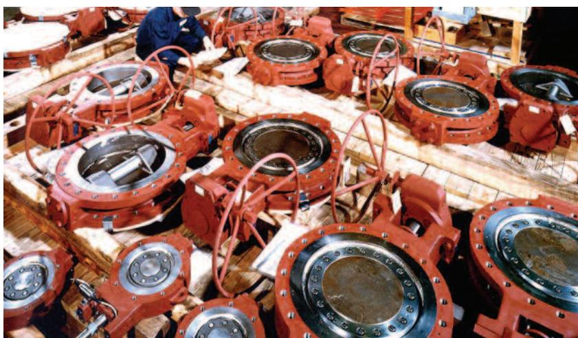
*Weir Valves & Controls TRICENTRIC metal seated butterfly valves for service water applications in the Lungmen ABWR in Taiwan*
