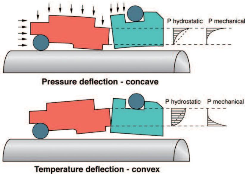
Figure 1: Typical seal face deformations
