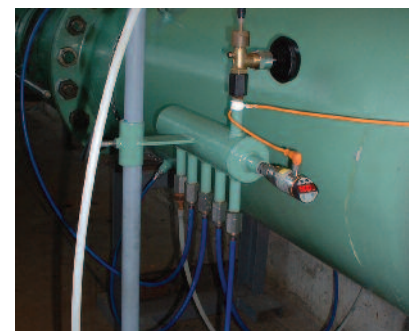
Figure 3: Pressure offtake point – collecting vessel with a vent valve and pressure gauge (p1)
