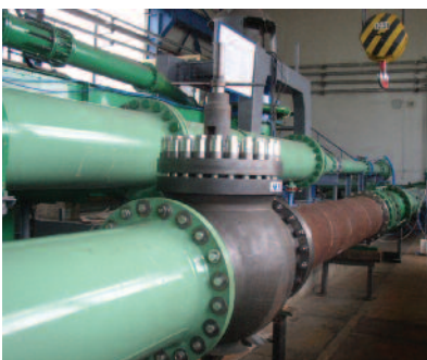
Figure 1: Swing check valve with disk position fixation in the test rig
