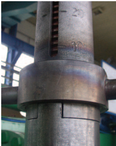
Figure 4: Means enabling mechanical fixation of position of the valve disk at a selected angle
