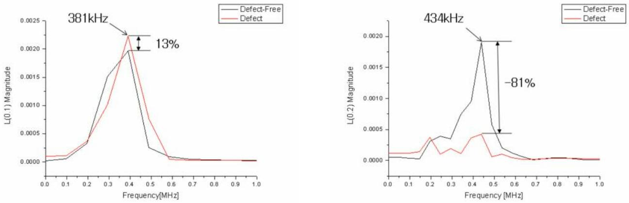
Figure 5. Signal characteristics of L(0.1) and L(0.2) mode on frequency spectrum (a) Frequency spectrum of L(0.1) (b) Frequency spectrum of L(0.2)
