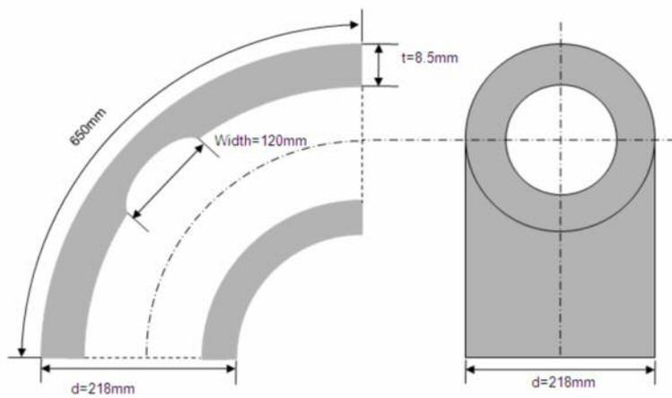
Figure 2. Shape of defects in 8.5mm thick elbows
