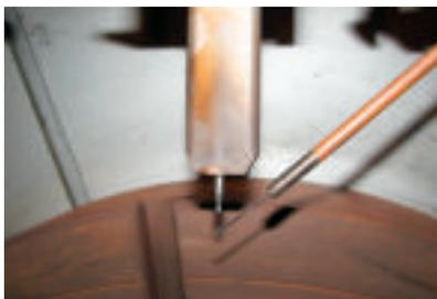
Figure 5. A narrow gap torch with hot wire tube showing the wire angle and position relative to the tungsten.
