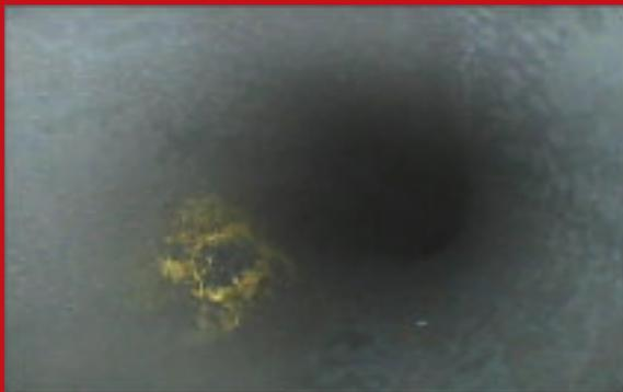
Figure 5. Borecope photo showing tube defect.
