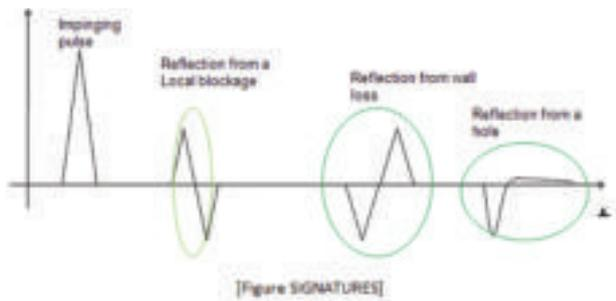
Figure 1. Different defects have their own particular acoustic signatures, enabling them to be distinguished from one another.
